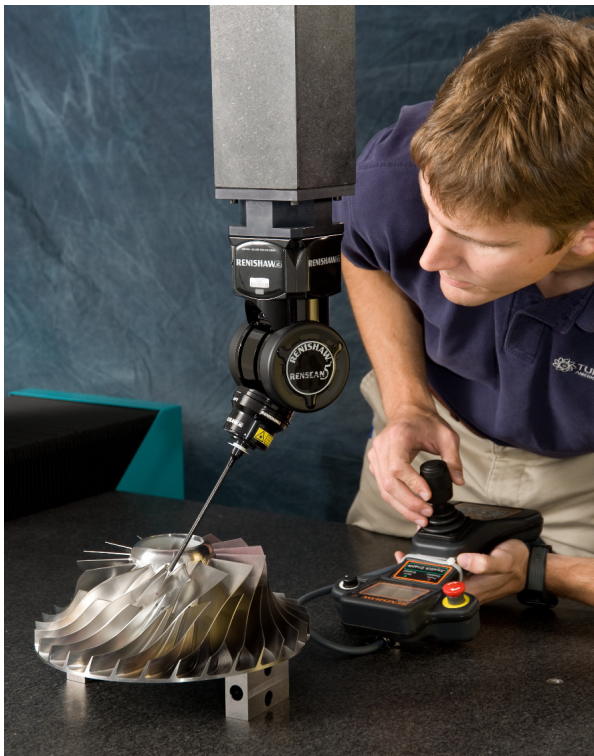
Nick Dean, TURBOCAM Product Engineer/CNC Programmer, uses teach points to create a five-axis program for inspection of a shrouded impeller
